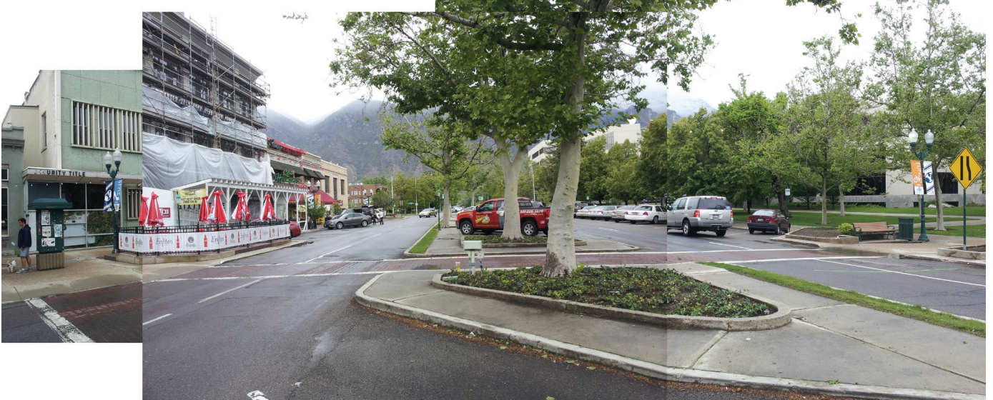
Center Street in downtown Provo with medians, bulb-outs, and diagonal parking.;
